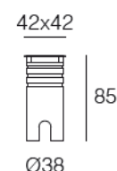
A00486_0 Recessed box in aluminum with edge (installation with aluminum trim)
